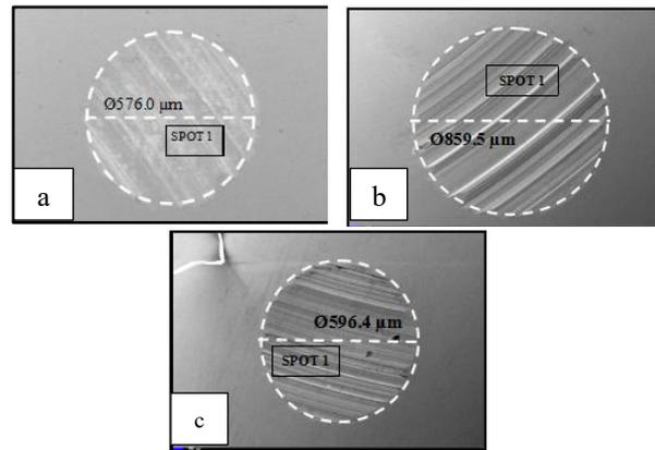
Figure 4 SEM micrograph of worn surfaces on a ball bearing under lubricated conditions of (a) sample 2, (b) Sample 4 and (c) optimized sample.
