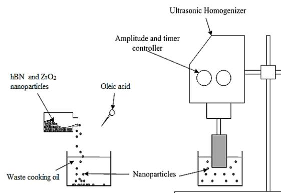
Figure 1 Schematic diagram sample preparation by using ultrasonic method [3].
