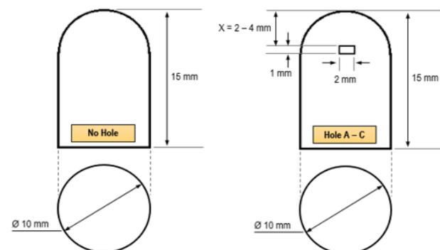
Figure 1 2D modelling of fabricated pins.
