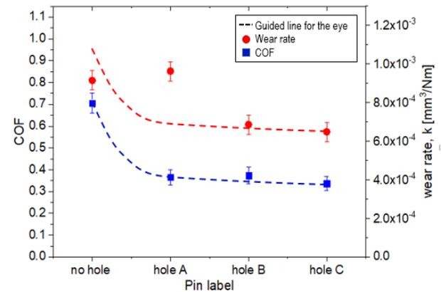
Figure 3 Friction and wear of 3D-printed pins.
