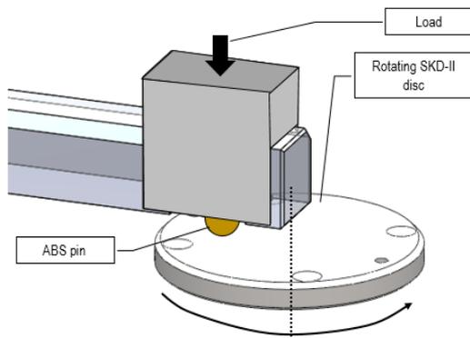
Figure 2 Schematic diagram of pin-on-disc test.
