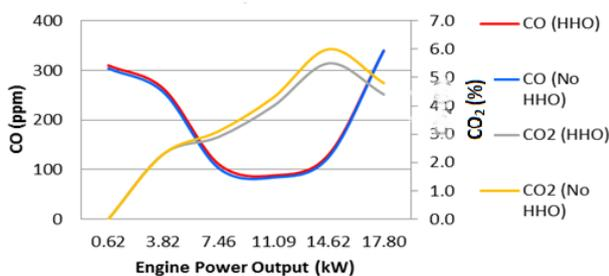
Figure 2 Changes in emissions due to HHO Generator use.
